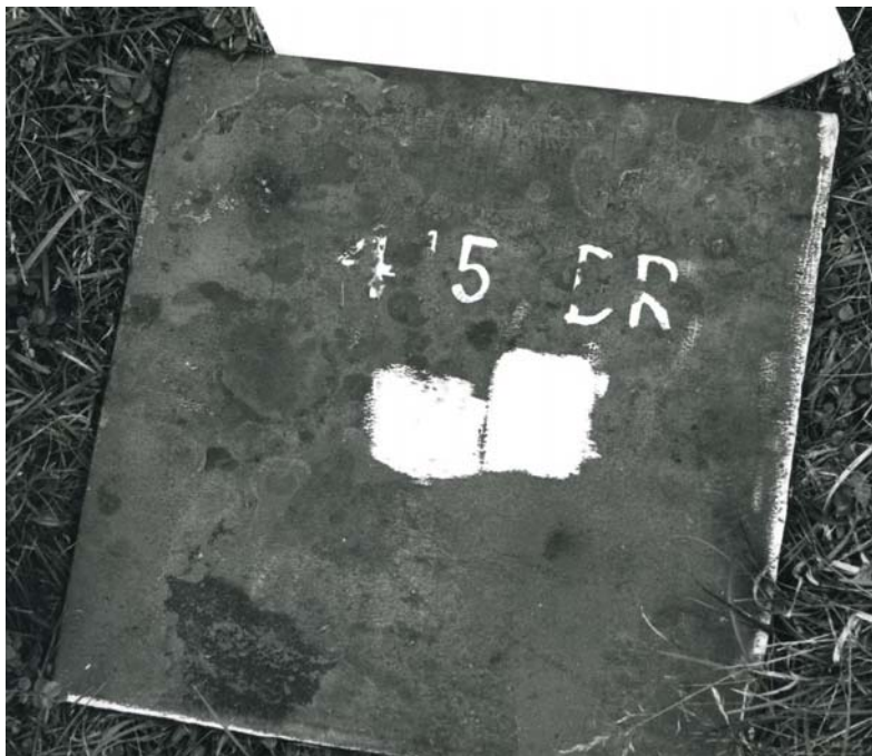
Plate of 415 Brinell Harness as used on the Shorland Mark 3. Viewed from the back showing no penetration.
