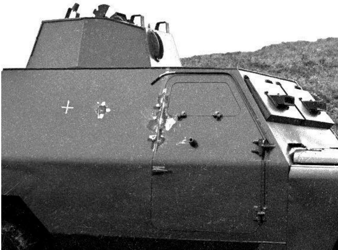
The Shorland Mark 3 showing the 50 metre strike to the right of the target cross & deliberate hits at the door edge (Photo via Geoff Fletcher)
